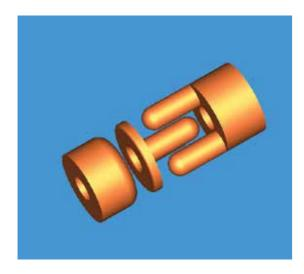
Figure 2.2a. Electrodes of accelerating period with spatially-periodic quadrupole focusing (RFQ DTL)
