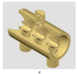
Figure 2.4. Main part of accelerator MPA-3 (CC DTL): Coupled Cavities
