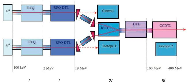
Figure 2.5. Structure of the linear accelerator
