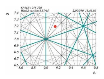
Figure 2.11b. Betatron tune plots and operating point.
