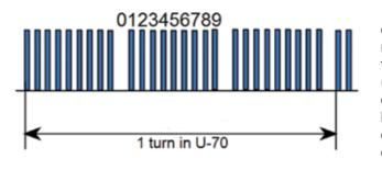
Figure 2.7. Beam structure in the U-70 with injection from the U-3.5
