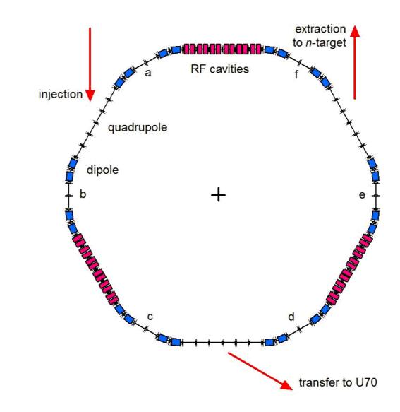
Figure 2.9. Layout of key technological systems of the U-3.5
