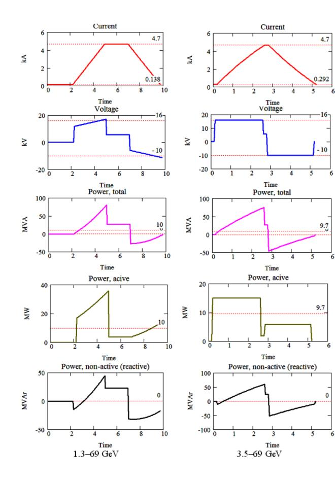
Figure 2.13: Electrical diagrams for a power supply convertor. Peak current is 4.7 kA.
