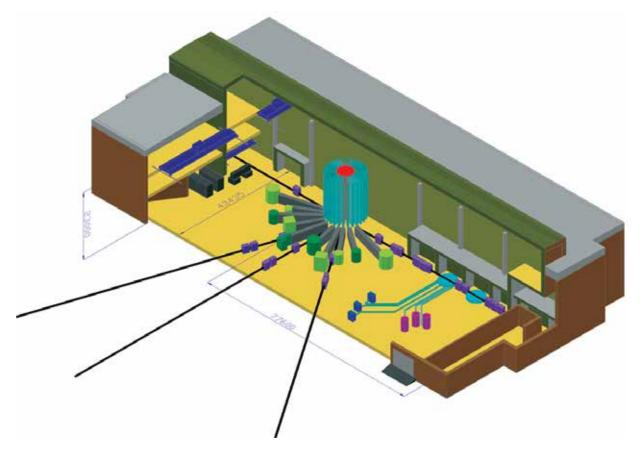
Figure 4.1. Layout of experimental hall with target, system of channels and facilities for experiments with thermal and cold neutrons.
